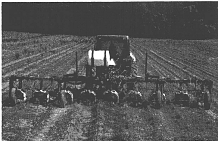
Figure 2. Eight-row sensor-controlled hooded sprayer in soybean field.
